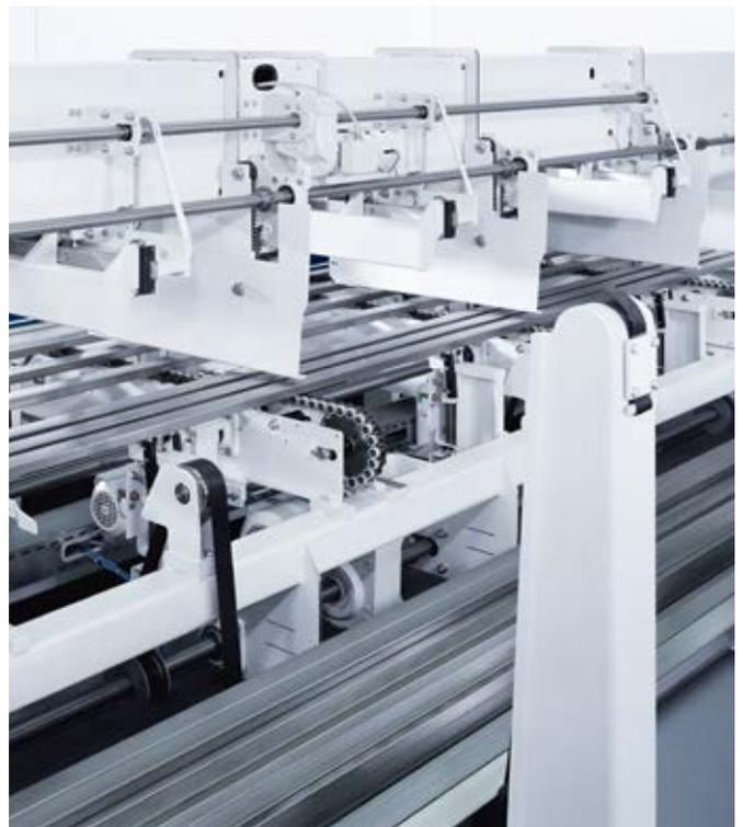
LoadMaster Tube for the TruLaser Tube 5000.
