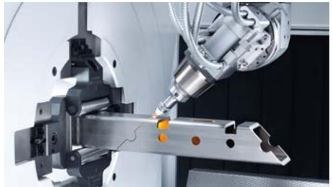
The bevel cut opens up new production possibilities.
